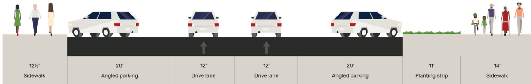
Figure 8. Section D (Kansas Ave to 4th Street) – Existing (64' curb to curb)
